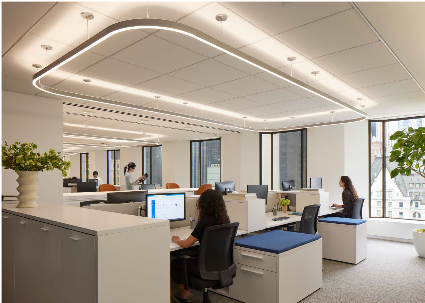
Installation of LED lighting is helping drive reductions in energy usage through efficient lighting, daylighting controls, and occupancy sensors.
